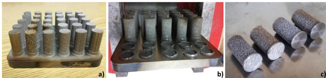
Figure 6. (a) test specimens after the thermal annealing process, (b) removal of specimens from the platform, (c) untreated and treated test specimen base.
