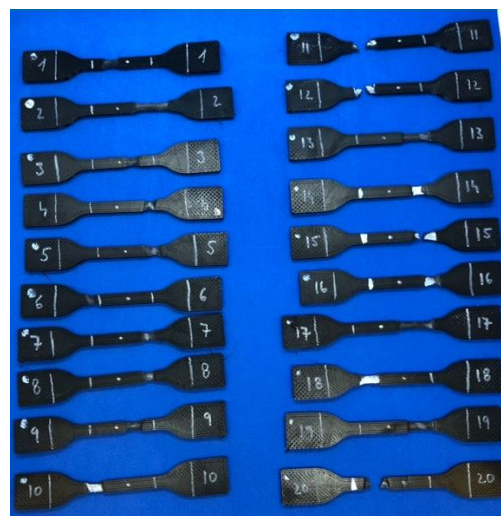
Figure 12. PETG samples after tensile test.
