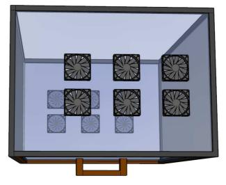
Figure 3a Laminar box design
