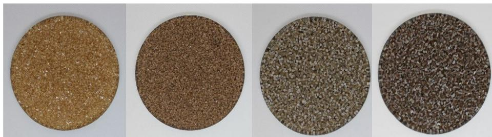
*Fig. 1 Pellet form of materials for extrusion (A: pure PPSU ; B: pure PEEK ; C: PPSU + HA/TCP ; D: PEEK + HA/TCP)*
