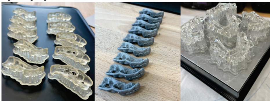
Figure 3: Surgical guides made by additive manufacturing a) Formlabs Form 3B b) HP Jet Fusion 5200 c) EnvisionTEC Vida
