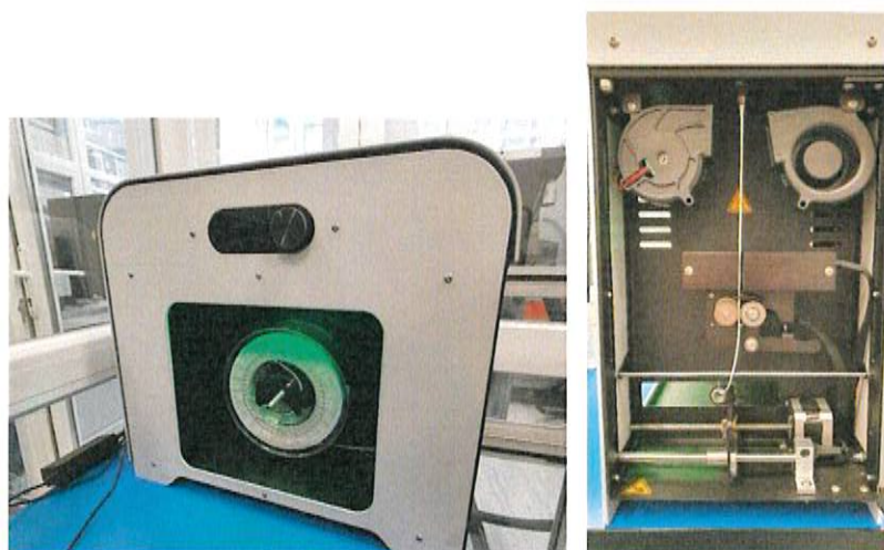
Figure 1. Extrusion process using the Filamentmaker - Composer series
