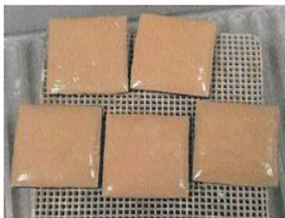
Figure 2. CoCr samples after last firing [own processing]
